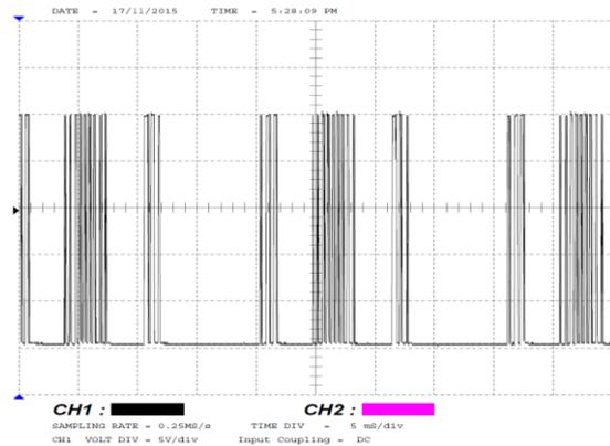
Fig.5. PWM signal for switch S1.
