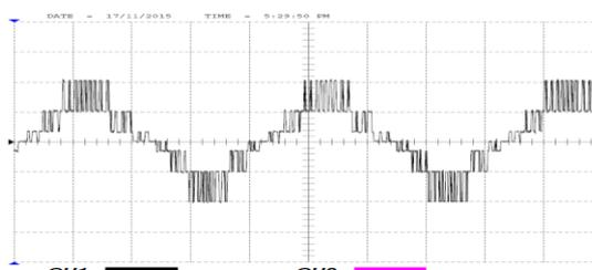
Fig.12. Output Voltage of seven level Inverter.
