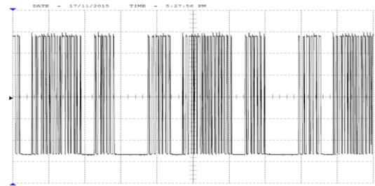
Fig.9. PWM signal for switchS5.
