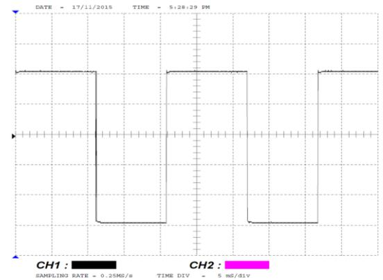
Fig.6. Pwm signal for switch S2.
