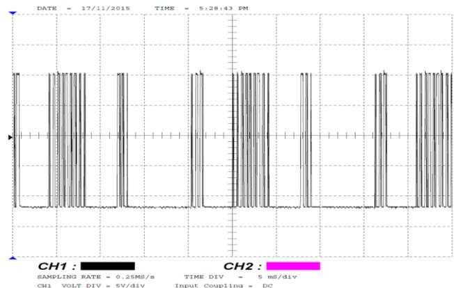
Fig.7. PWM signal for switch S3.
