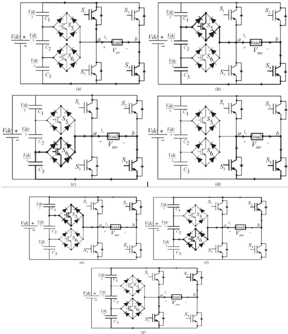
Fig. 2. Seven switching combination required to generate the output voltage (Vab).
