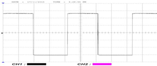
Fig.8. PWM signal for switchS4.
