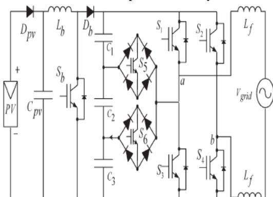
Proper switching of the inverter can produce seven output-voltage levels ( $V_{dc}$ ,  $2V_{dc}/3$ ,  $V_{dc}/3$ ,  $0$ ,  $-V_{dc}$ ,  $-2V_{dc}/3$ ,  $-V_{dc}/3$ ) from the dc supply voltage.
